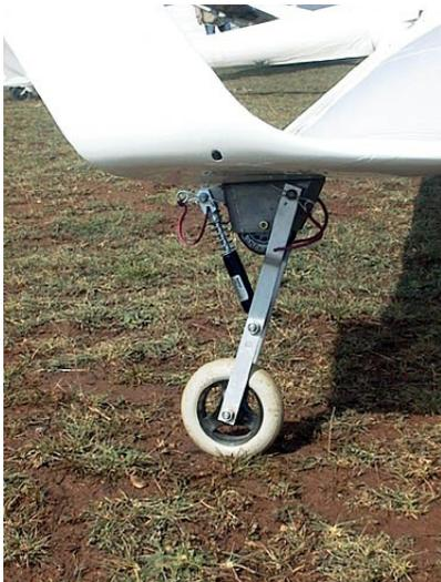
Taxiing on rough or soft ground may not be practical with the usual small wing tip wheels. Using a larger temporary tip wheel can save the day, though it must be removed before flight. DG Sailplanes makes one that can be folded and stowed in the baggage area after removal.
