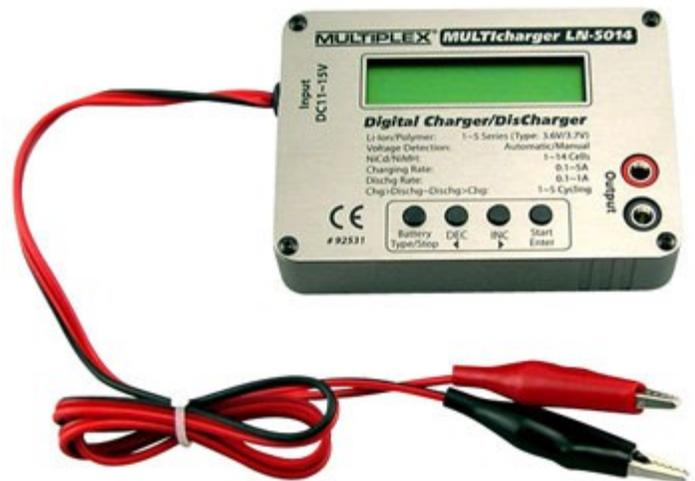
I use it with a 12 volt, 12 or 18 amp-hour battery to power my charger. After a flight, and the glider is tied down, I'll connect the charger to the glider and start charging. By morning, with the glider completely charged, I'll place the charger and it's battery in the trailer, so the battery has all day to charge from the trailer's solar panel before I need it again in the evening.
