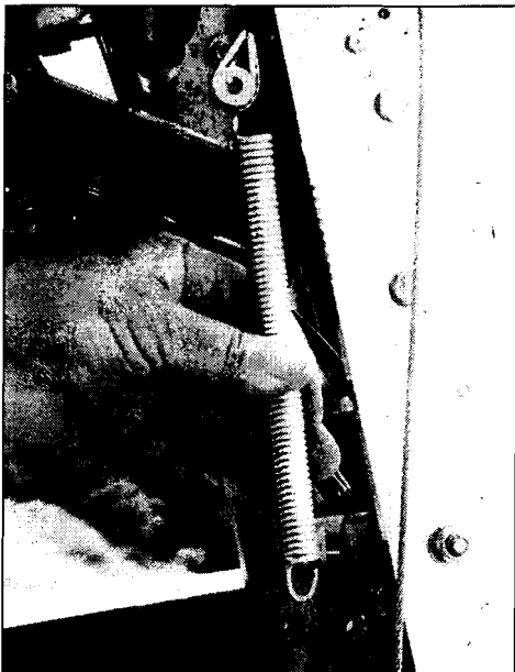
Tension Spring on Grob TWIN S/L. McGhie photo
